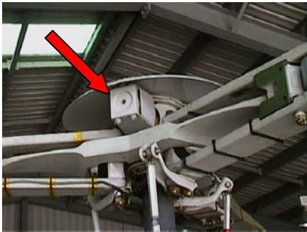
AS350 head mounted damper
